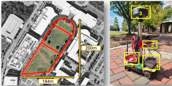
Fig. 4. Target environment, data collection path, and data acquisition vehicle.
